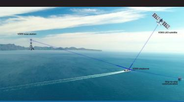
SAAB Transpondertech provides communication via VDES to ensure enhanced maritime safety (bandwith 32 times higher than AIS). Share information with other ships based on the VDES standard (IEC 2092-1)
